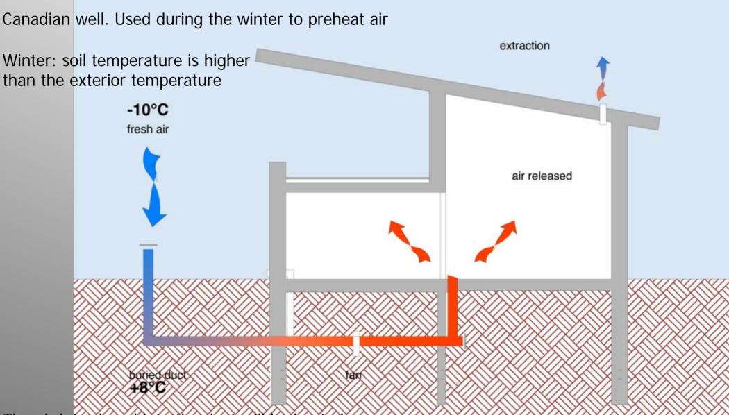
The air introduced into the duct will be heated
