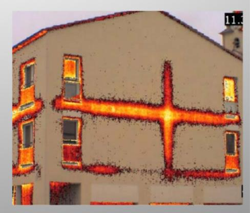
Thermal bridges are points or linear areas of construction where the insulating barrier is broken
