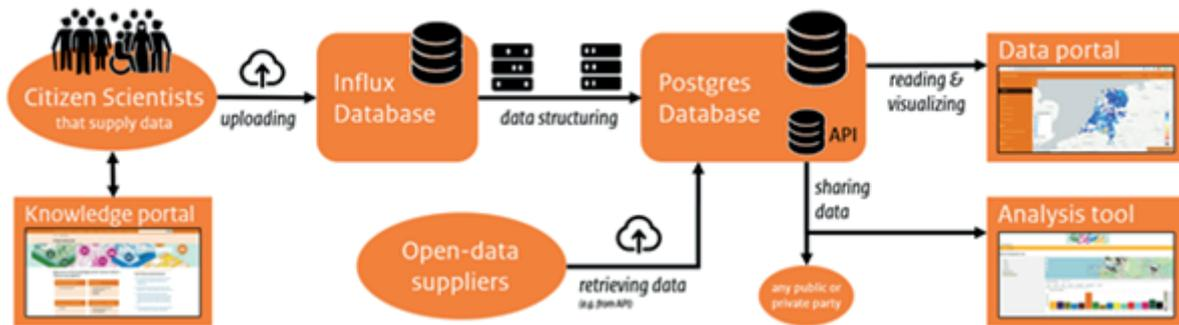
Figure 8: Diagram of the Measure Together infrastructure.
