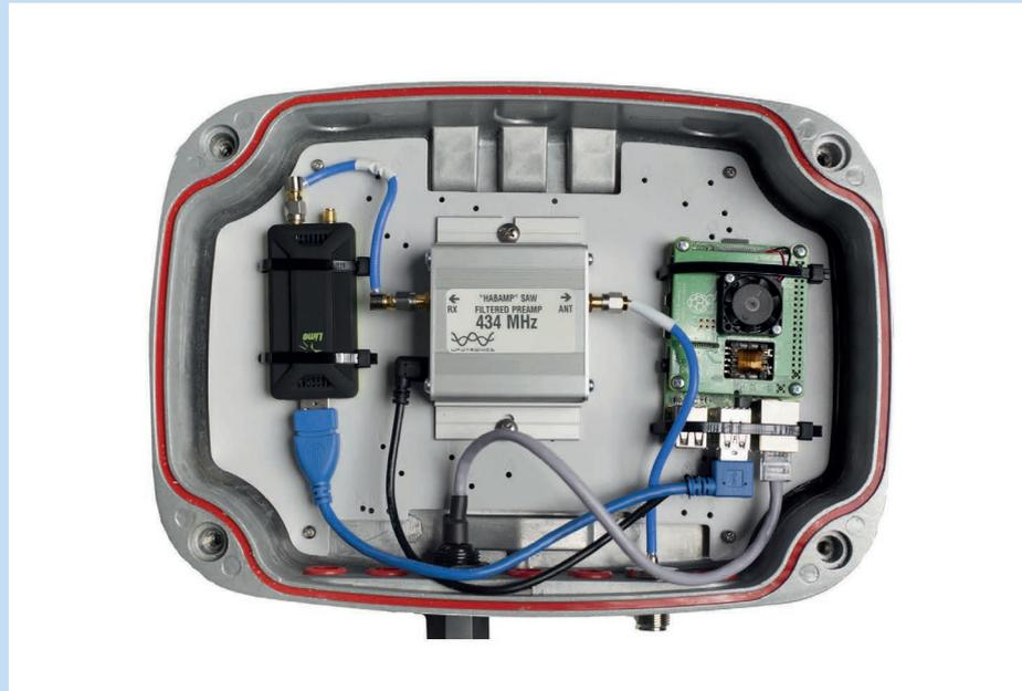
**Figure 13:** View of interior of ground station transceiver. Source: *LSTN Handbook*
