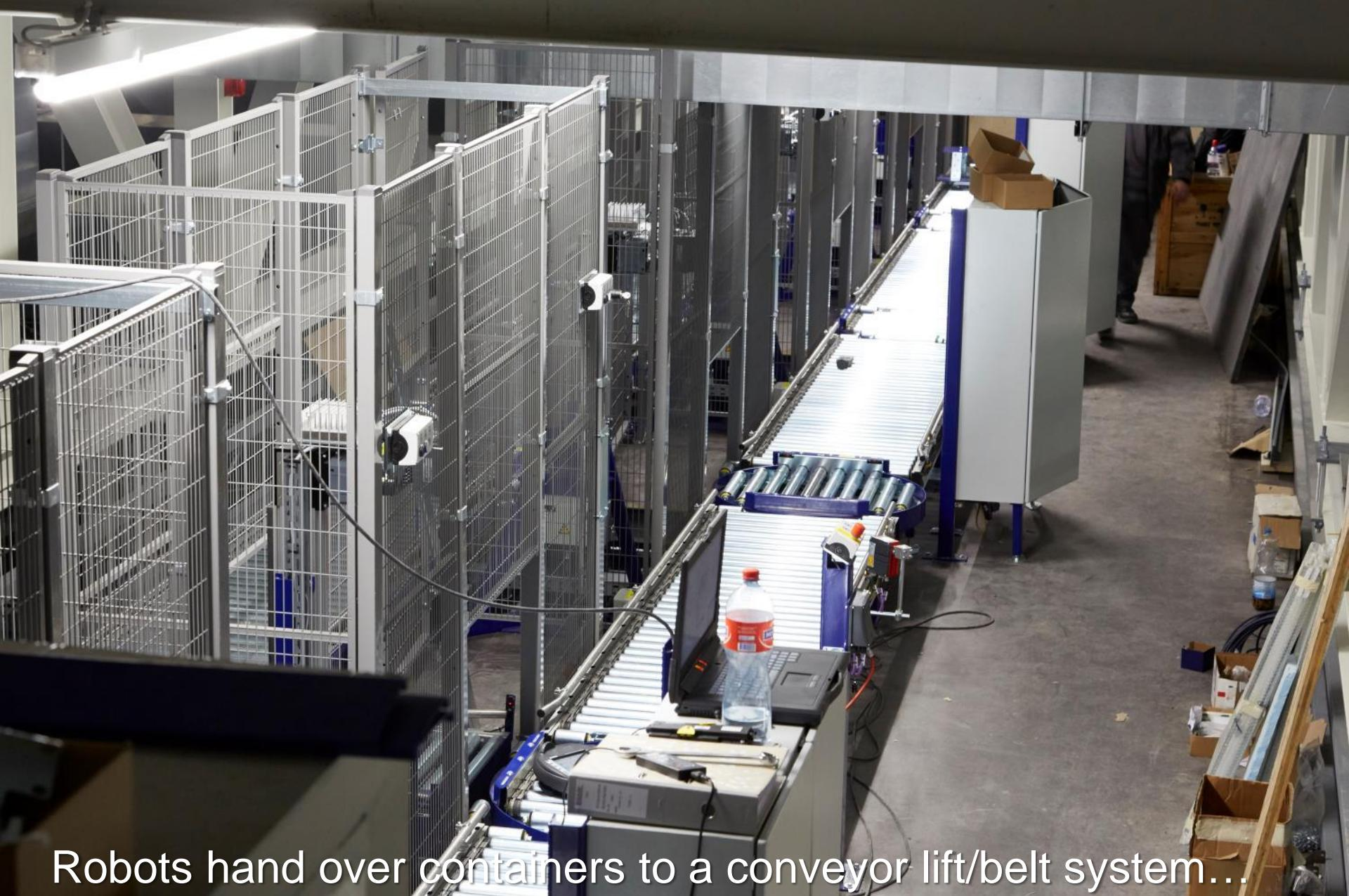
Robots hand over containers to a conveyor lift/belt system...
